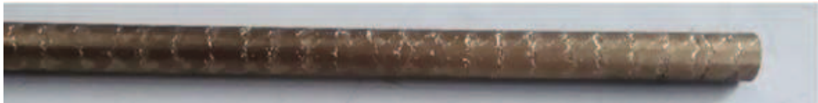
Figure 1. Photograph of CuAlMn shape memory alloy bar \varnothing 8 mm after casting
