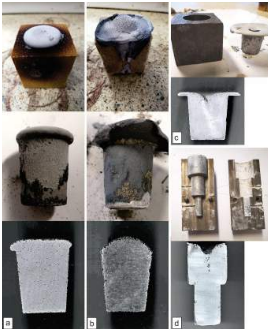
Figure 7. Castings from: Croning mould (a), CO 2 mould (b), graphite mould (c) and steel mould (d)
