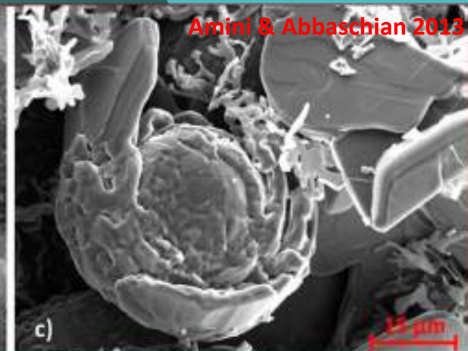
circumferential growth in a Ni-C alloy
